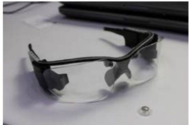
Figure 3: Innovega combines a contact lens with smart glasses that project images onto the lens.
